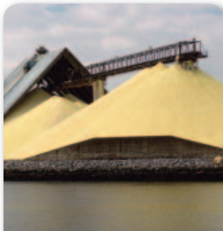
■ Figure 11.9 Sulfur, such as these piles at Vancouver Harbor, can be extracted from petroleum products by a chemical process. Sulfur is also mined by forcing hot water into underground deposits and pumping the liquid sulfur to the surface.
