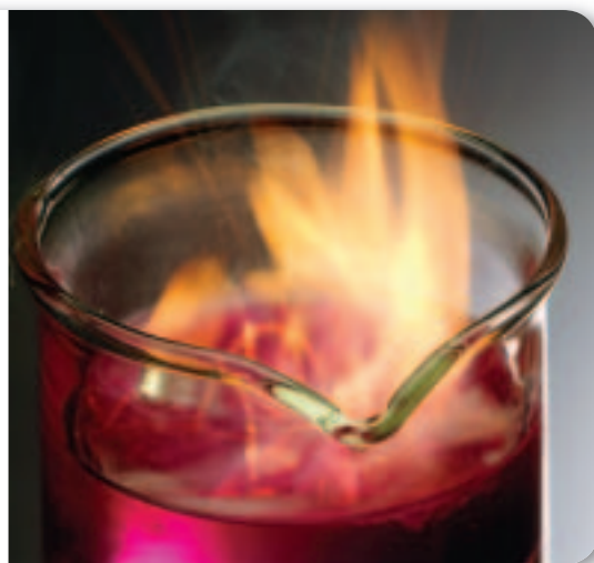
■ Figure 11.3 Potassium metal reacts vigorously with water, releasing so much heat that the hydrogen gas formed in the reaction catches fire.
